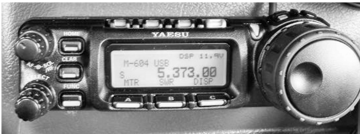
An example of one of the four long-range transceivers used by the W6JUL team.
